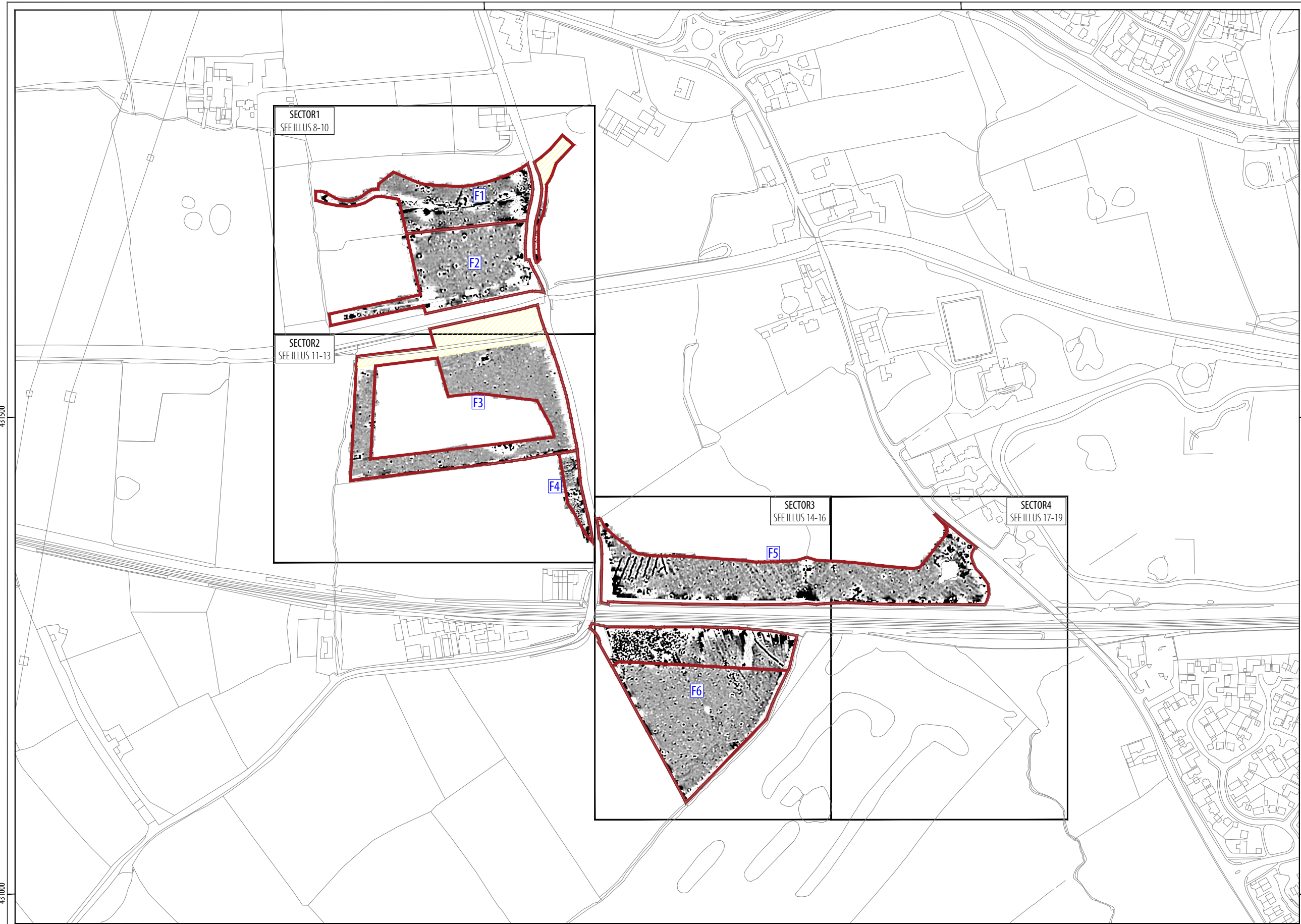
ILLUS 6 Processed greyscale magnetometer data
