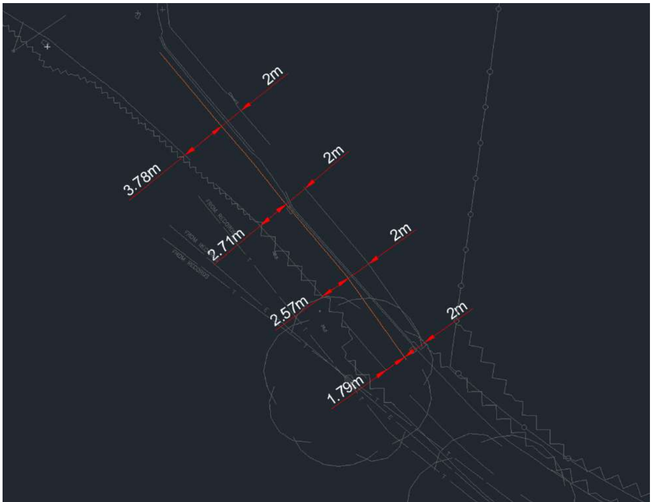
Figure 6.1 : Stoney Lane Dimensions (based on Topographical Survey)
