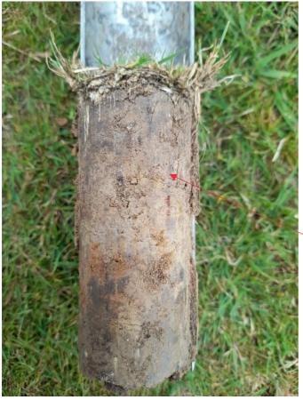
Good quality clay loam visible down to a depth of (100mm) over the indigenous sand based loam, with traces of grit.
