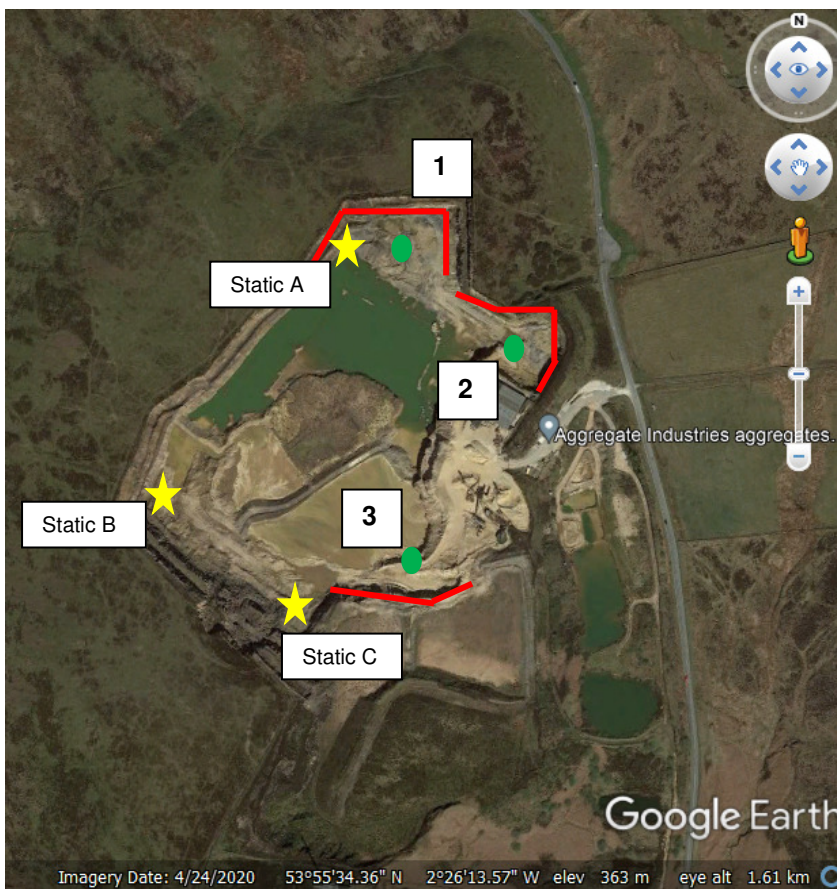
Plate 2. Quarry rock faces subject to survey (red lines) and corresponding position of surveyors (green circles 1-3) and static detectors (yellow stars A-C) during the 2021 surveys.
