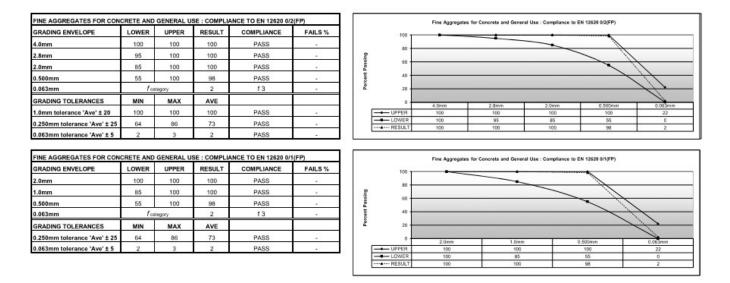
The option exists to blend crushed sands from the sand and gravel deposit with the Upper Sand thereby increasing resources of high-quality BS EN 12620 0/4 (MP) concrete sand.
