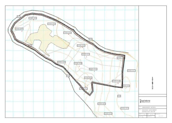
The extraction batter has been set at 25m standoff from the River Ribble and with an overall slope profile of 1v in 2.5h. The brown contours represent the topography and the grey contours represent the base of mineral workings.
