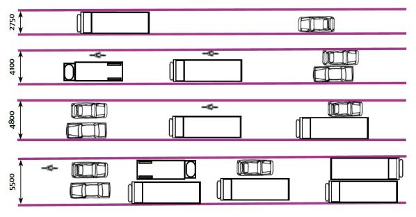
A carriageway of 5.5m can accommodate two-way HGV movements, however, this is on a straight and has minimal clearance between vehicles. Where bends exist greater widths of carriageway would be required. Further, the above does not factor in the needs of pedestrians as it assumes footways adjacent to the carriageway would be available.
