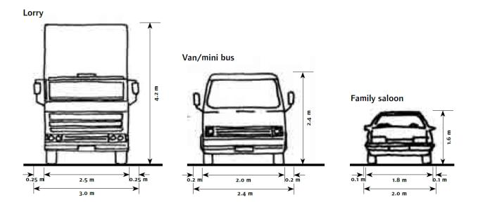
Figure 7.1 from MfS, reproduced below, shows what carriageway width can typically accommodate.
