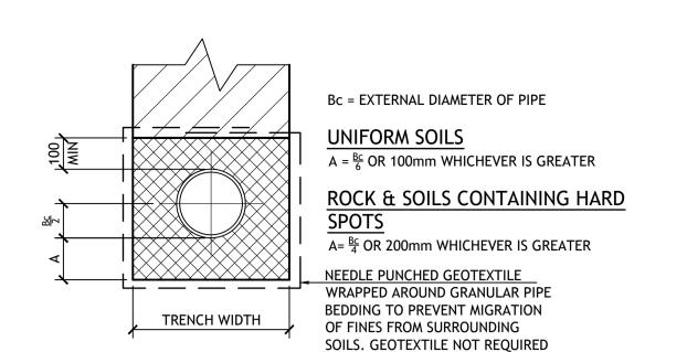
IN COHESIVE (CLAY) MEASURES MAIN BACK FILL SELECTED EXCAVATED MATERIAL. COMPACTED IN LAYERS NOT EXCEEDING 225mm. IN COHESIVE SOILS TRENCHES UNDER ROADS AND HARD STANDINGS SHALL BE BACK FILLED WITH IMPORTED GRANULAR MATERIAL.
